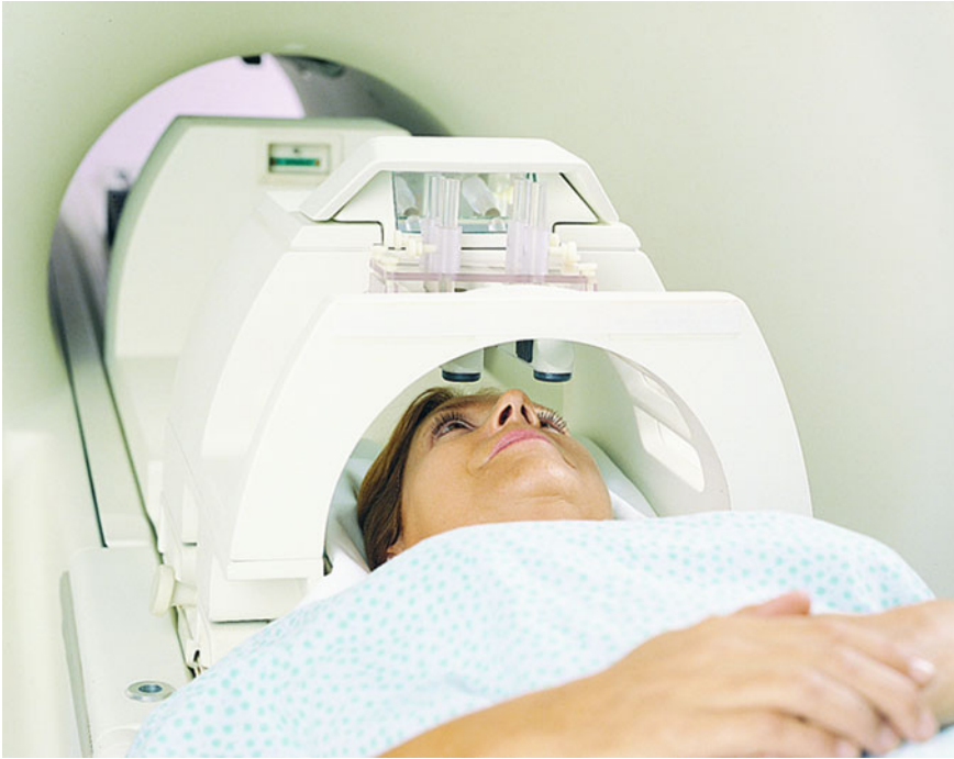
Fig. 21.1 Example of eye tracking fMRI scanner. Courtesy of SensoMotoric Instruments (SMI), Needham, MA http://www.smiusa.com . Reproduced with permission
