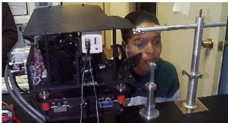
Fig. 5.9 Dual-Purkinje eye tracker. Courtesy of Fourward Optical Technologies, Buena Vista, VA ( http://www.fourward.com ). Reproduced with permission
