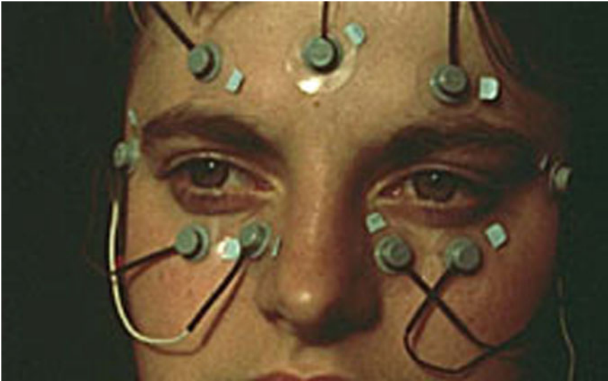
Fig. 5.1 Example of electro-oculography (EOG) eye movement measurement. Courtesy of Metro-Vision, Pénarchies, France ( http://www.metrovision.fr ). Reproduced with permission
