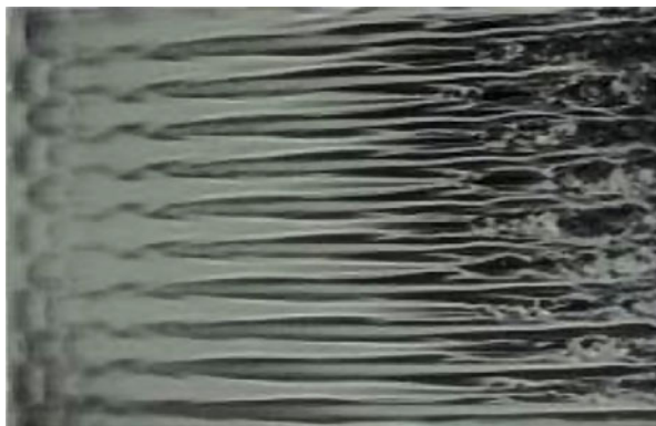
Fig. 6.14 Streaks as a consequence of the lift-up effect in a Blasius boundary layer. The flow is from left to right . Note that the disturbance generating the streaks is characterized by a spatial periodicity in the spanwise direction and that the streaks are themselves unstable at some downstream position (Photo by Elofsson and Matsubara, in Elofsson 1998)
