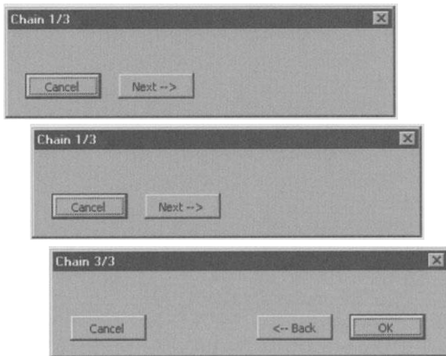
Figure 7.29. A three-stage chain of forms (only one form at a time is visible)
