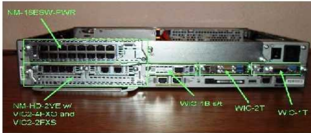
Figura 21 – Cisco 3700 Series multiservice-access-router Interfaces .
