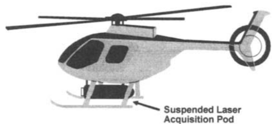
Figure 5-1. Suspended Laser Acquisition Pod. The SLAP system is housed in the aerodynamic shell below the helicopter fuselage.
